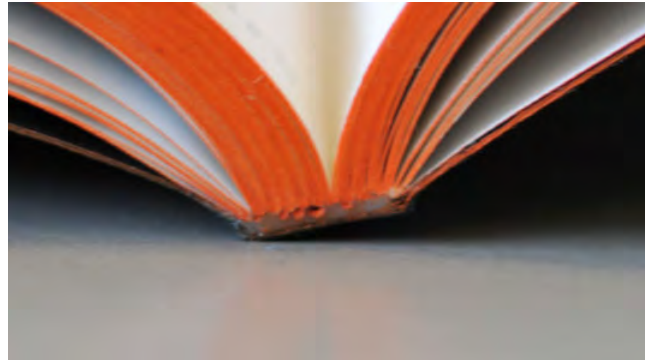
Figure 10: Perfect Binding with Sewed Hotmelt
