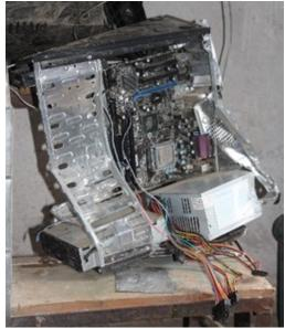
Figure 11. School computers and lab supplies were damaged where no non-structural mitigation measures had been taken. Photo: R. Paci-Green/Risk RED
